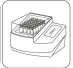
Seal the vials in the preheated thermoreactor for 120 minutes at 150 °C.
