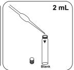
Prepare two reaction vials. Put 2 mL deionised water Put 2 mL sample in the in the blank.
